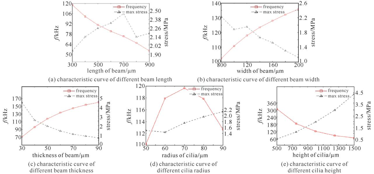
Fig. 5 Characteristic curves of different microstructure sizes
