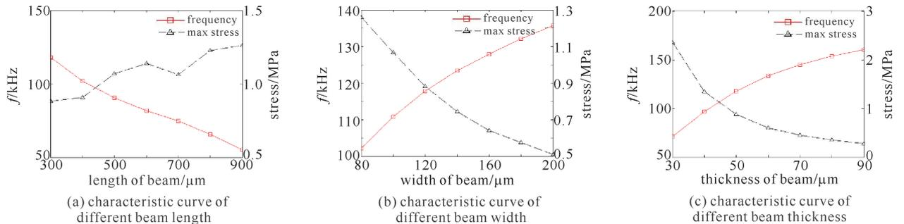
Fig. 6 Characteristic curves of different cantilever beam sizes
